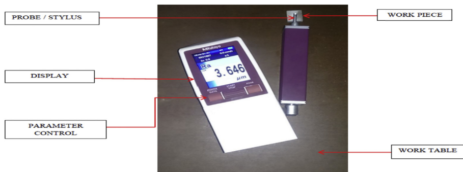
Fig. 7. Surface roughness measurement.
