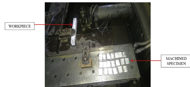
Fig. 3. Work material mounted on WEDM machine.
