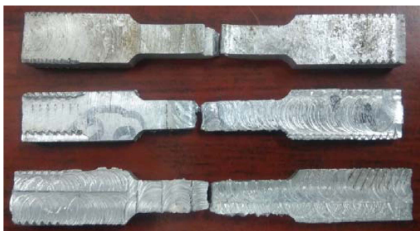
Fig. 8. Fractured surfaces of hybrid composites.
